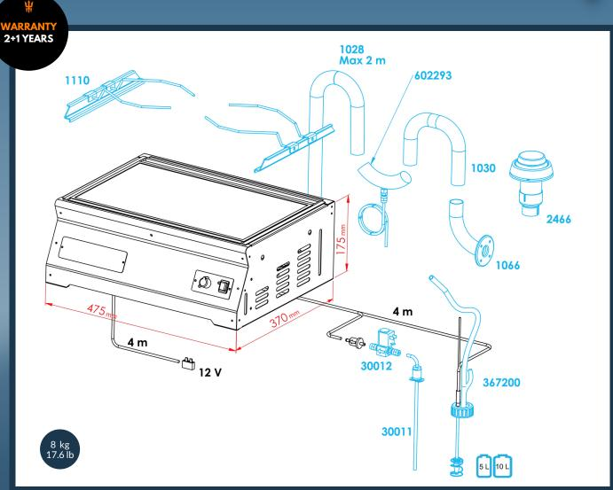
Accessories in black come with the standard package. Accessories in blue are additional. The calculated values are measured in a reference measurement wall, which is constructed to respond to a typical boat installation. The technical values have been measured with the maximum length of ducting, exhaust pipe, fuel line, and power cord. The figures allow for 10 % reserve - yours may vary.
